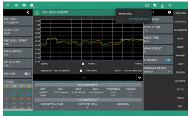
EMF results show power from each antenna axis and summary results for peak and average power over a defined time period
