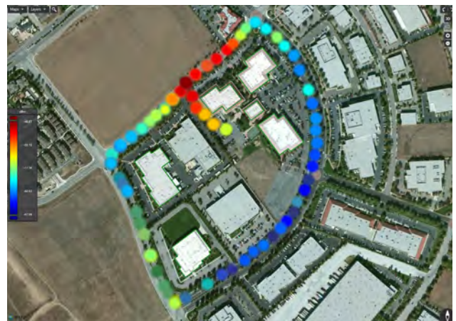
Typical result screen for outdoor coverage mapping
