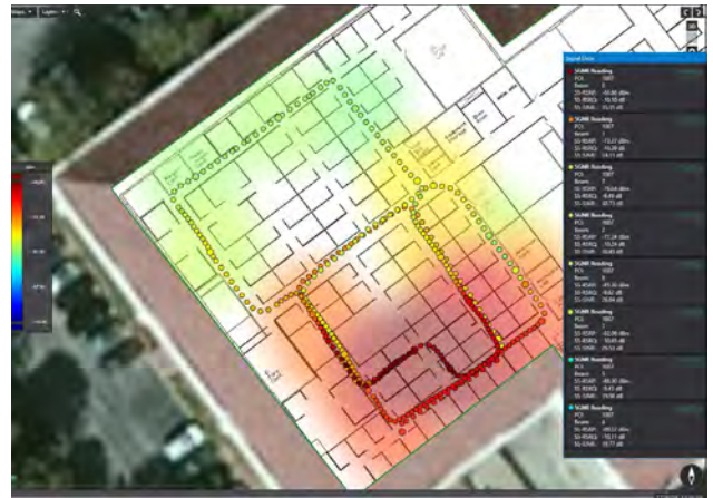
Typical result screen for indoor coverage mapping
